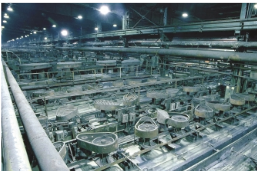
Banks of flotation cells at Norilsk Nickel's Talnakh operation on the Taimyr Peninsula in Siberia.
