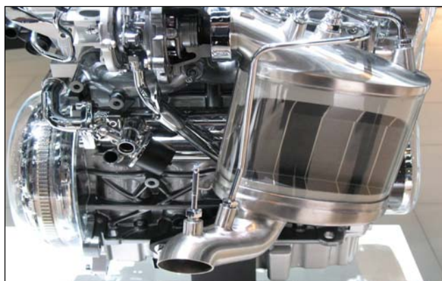
Above: Cutaway view of a catalysed soot filter (CSF) mounted directly on the turbocharger of a passenger car diesel engine (Image copyright Martyn V. Twigg)
