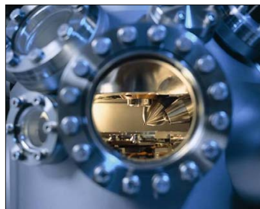
Above: Close-up of the analysis chamber of the ION-TOF GmbH Qtac 100 low-energy ion scattering instrument
