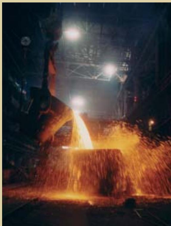
Pouring molten copper-nickel matte at Norilsk Nickel's Nadezhda smelter.
